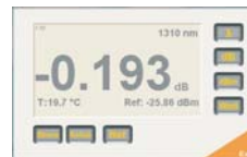
OPL5 Power Meter application with datalogging
