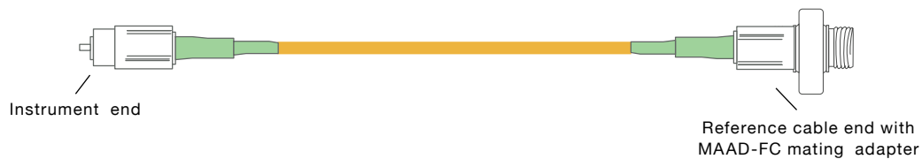
Figure 1: SAVER cable overview
