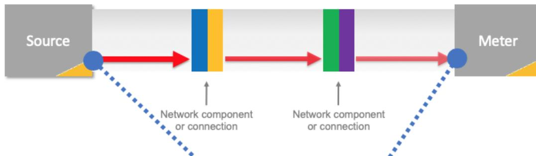
$$IL = 10 \text{ Log (transmit power / receive power)}$$
